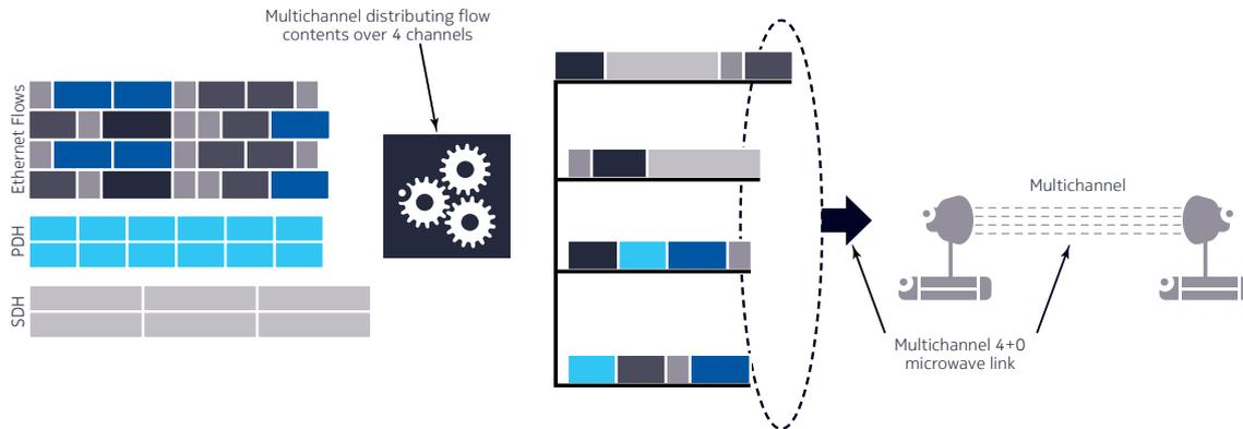
Because the Nokia 9500 MPR transports all services in a packet format (that is, traditional TDM and ATM services are packetized) it can take full advantage of an adaptive modulation aware multichannel capability:
