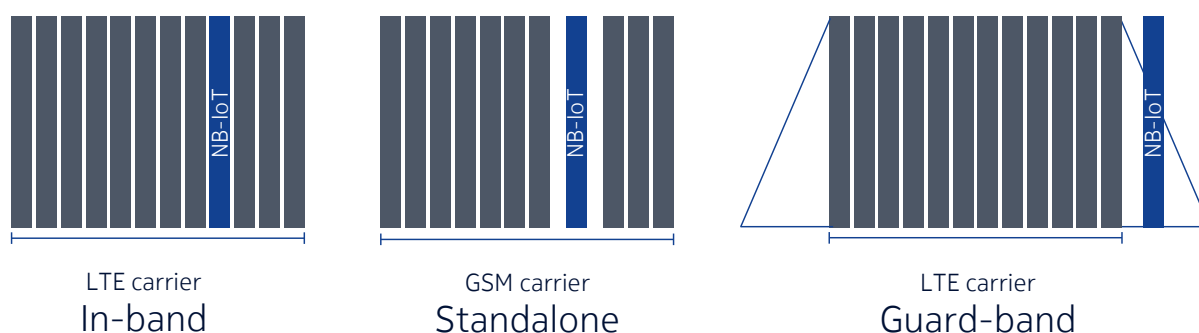
Figure 5: NB-IoT deployment options
