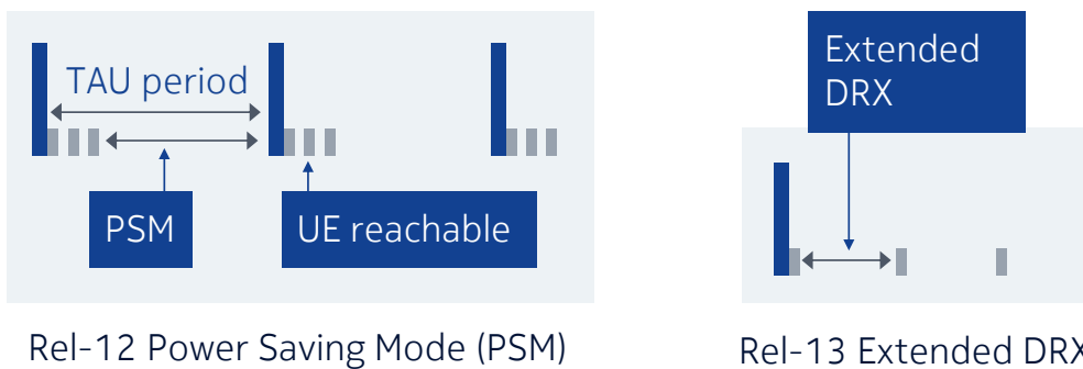
Figure 6: LTE-M/NB-IoT enhanced battery options
